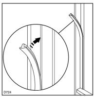
Apply covers (C-D) on joint cover lugs and into hinge holes.
